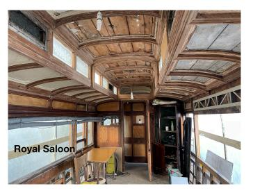
train at a cost of £40,000, a royal sum, even in those days. Currently the job of the moment, as of January 2023 we have stripped the wood of paint (thanks to Dave's Dad John!) Repair work has begun on the frame and our next task is to make the roof watertight.
